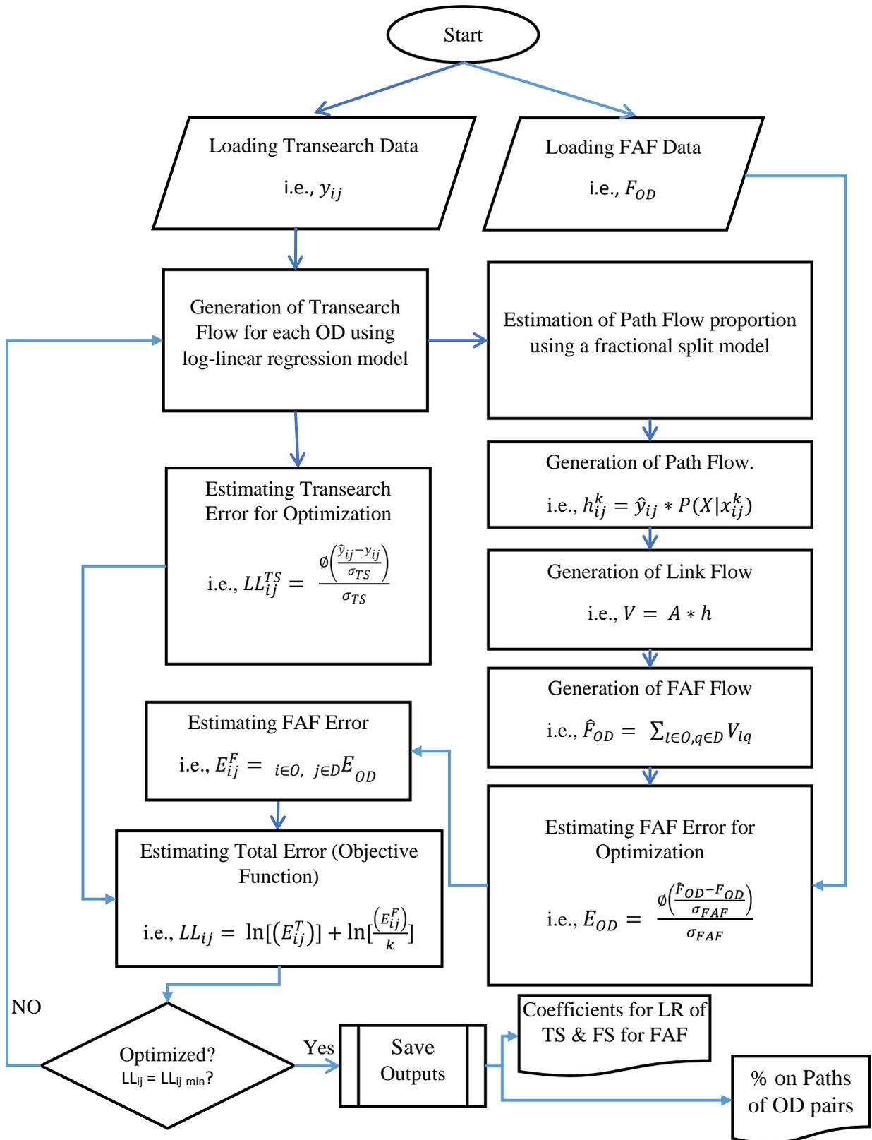
Figure 4-43: Flow Chart of Algorithm
